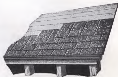
The above illustration shows Individual Slate-Surfaced Shingles laid over dressed and matched tight roof sheathing.
